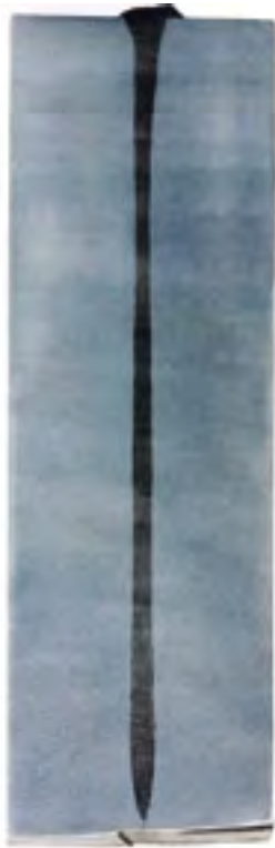
Typical deep welding in bronze/steel (30 mm, upper photograph) and aluminum (150 mm, lower photograph)
